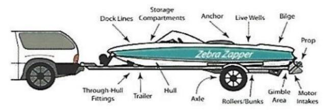
DRAIN water-related equipment (boats, ballast tanks, portable bait containers, motor) and drain bilge, livewell and baitwell by removing drain plugs before leaving a water access or shoreland. Keep drain plugs out and water draining devices open while transporting watercraft.
